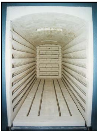
Insulating Fire Brick (IFB) Lining
